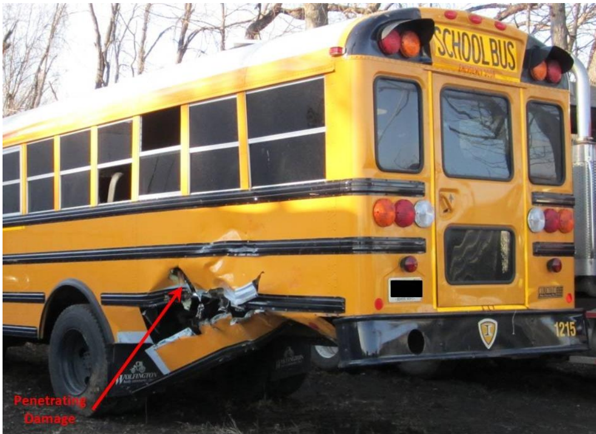
Figure 12. Damaged left side of school bus.
